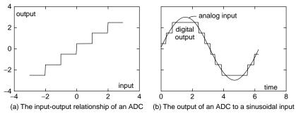
Figure P1.10 The characteristic of an ADC (analog-to-digital converter).
