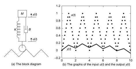
Figure P6.4 A mass-spring-damper system.
